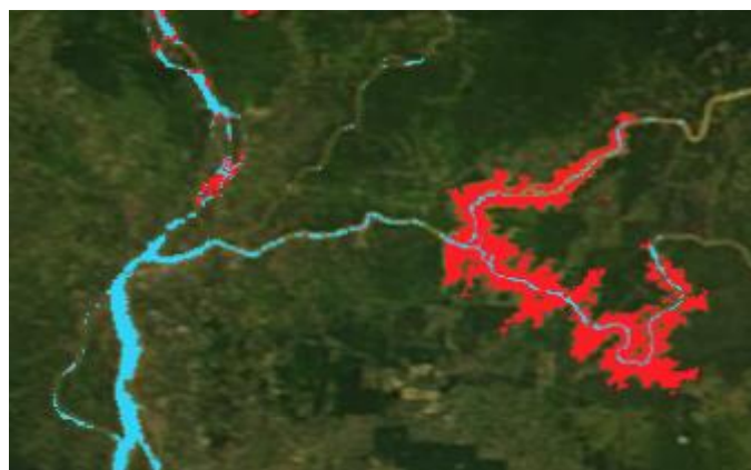
Figure 11: Example: New reservoir behind recently constructed Lower Sesan II dam in Cambodia misidentified as flood. 2-Day product, 24 Nov 2020, Worldview display.
