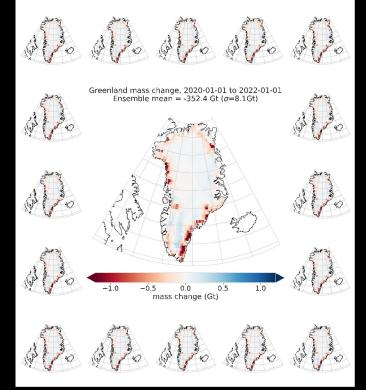
Greenland mass change derived from ICESat-2 ATL15 data and corrected for firn air content change, estimated from the firn model ensemble. Center panel is the ensemble mean, and surrounding panels are ensemble members (16 members).
