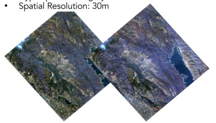
DESIS L2A (right) surface reflectance and L1A (left) top of atmosphere reflectance RGB thumbnails
