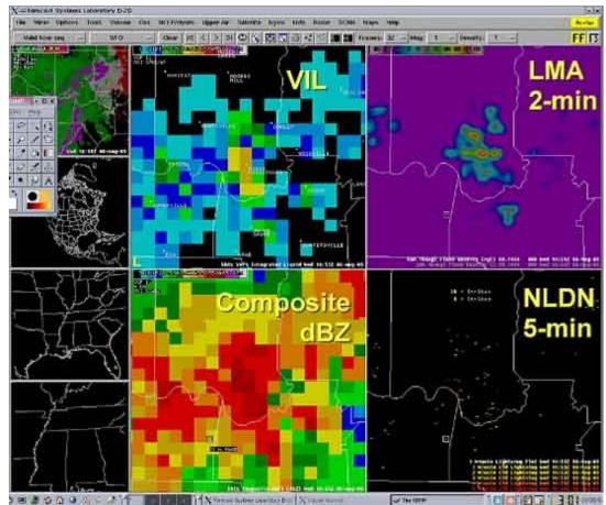
Weather forecasters rely on the Advanced Weather Interactive Processing System (AWIPS) display. This AWIPS includes Lightning Mapping Array (LMA) data (upper right corner) as a single gridded graphic showing lightning flash density. The display also shows National Lightning Data Network (NLDN) data, vertically integrated liquid (VIL) measurements, and radar reflectivity composites. (Courtesy SPoRT)
