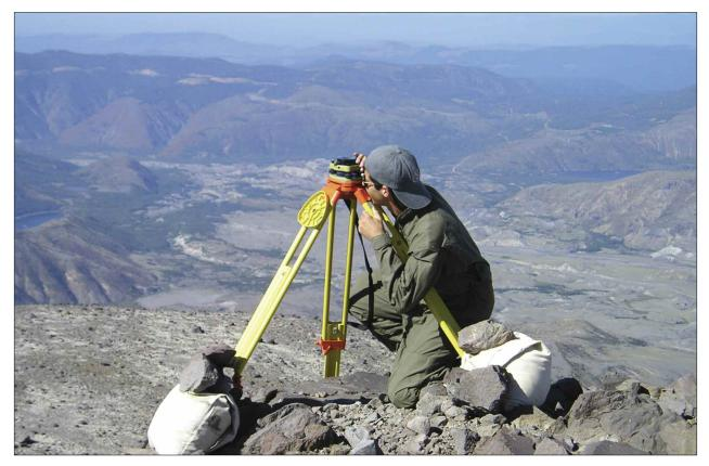
A researcher checks the calibration of a ground-mounted Global Positioning System (GPS) station on Mount St. Helens. GPS receivers and satellites can precisely capture movements in the Earth's crust, giving scientists a picture of processes concealed deep in the ground during earthquakes and volcanic eruptions. (Courtesy M. Lisowski)
