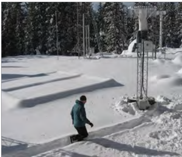
Snow telemetry (SNOTEL) sites are equipped with meteorological instruments that help scientists gauge the mountain snowpack. The rectangular shapes on the ground are snow pillows that estimate the water equivalent of the snow. (Courtesy A. Slater)
