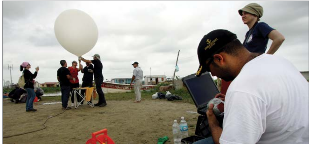
The team works to deploy a weather balloon with sensors attached to measure temperature, relative humidity, and pressure. (Courtesy H. P. Díaz/Centro de Modelado Científico)
