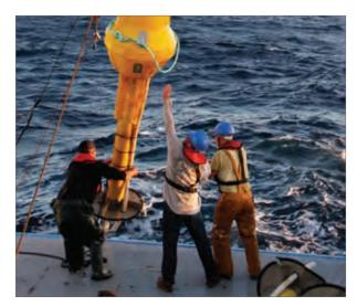
Crew onboard the *Thetys* research vessel recover Marisonde drifting buoys from the northwestern Mediterranean Sea. The buoys collected sea surface and air measurements for an oceanographic campaign in May 2013. (Courtesy M. Herrmann)
